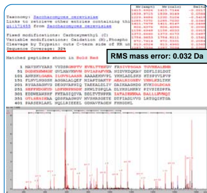
Fig. 3: DB search result of a nanoLC run with ETD-MS/MS of a 5 fmol Enolase tryptic digest (top). Sequence coverage is 32% with excellent data quality (bottom).
