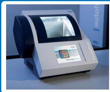
Fig. 1 ImagePrep station for push button matrix application to tissue sections. 20 \mu\text{m} droplet size for high resolution MALDI images.
